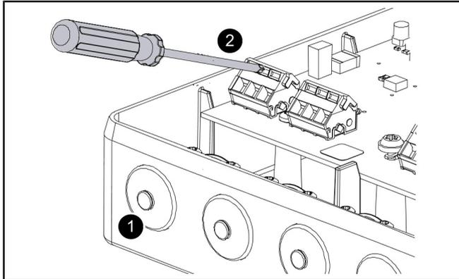
👁 Lay the connection cable securely (e.g. conduit pipe) from the system tank to the control unit. Ensure that there is adequate cable length for the maintenance of the electrical components.
